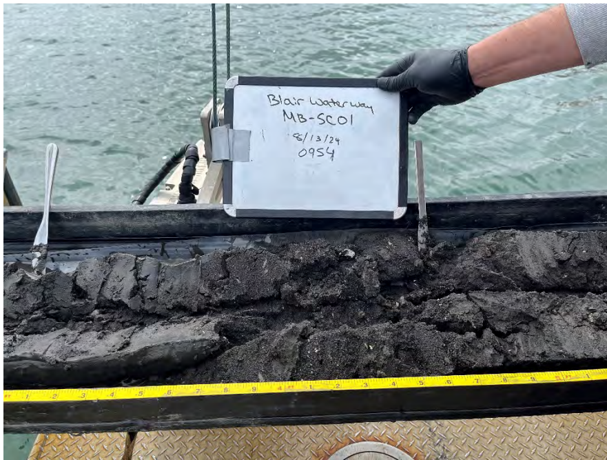
Photograph 4 MB-SC01 3.1 to 5.2 feet
