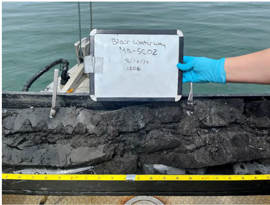
Photograph 11 MB-SC02 2.5 to 4.5 feet
